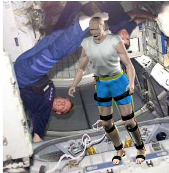
FIGURE 23: A Graphic View of the MEMICA-Based Exoskeleton for Countermeasures.
