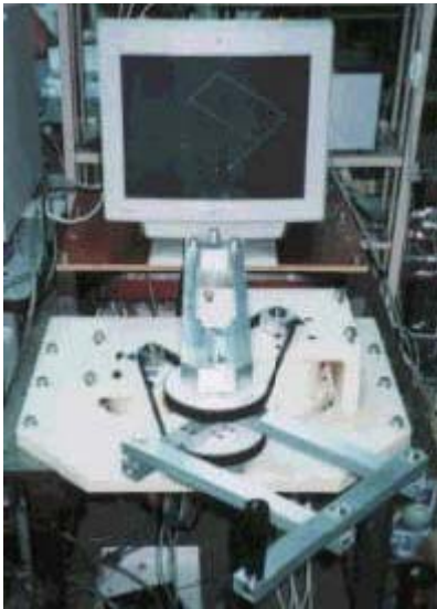
FIGURE 21: Force Display Device Using Electrorheological Fluids [Human-Machine Interaction Subarea website]. [Picture requires Permission]
