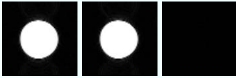
Fig. 13. Phantom scans with the interface at rest (left) and moving (center). The difference (right) shows neither shifts nor deformations.
