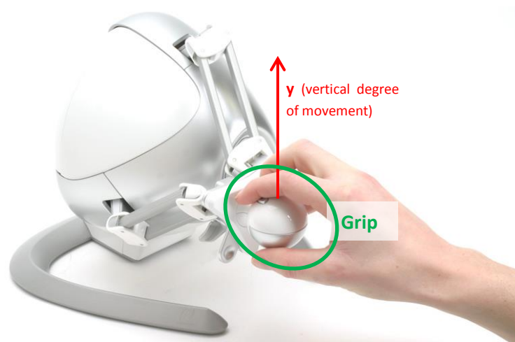
Figure 3.2: Novint Falcon haptic interface. The grip of the device, and the vertical degree of freedom, are indicated. (Figure taken from: bit-tech.net).
