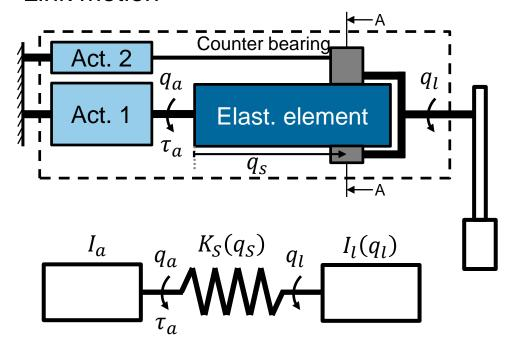
$$I_{l}\ddot{q}_{l} + G_{l}(q_{l}) + K_{s}(q_{s})(q_{l} - q_{a}) = 0$$
